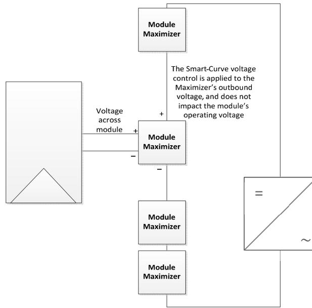
Figure 2: Block diagram of Maximizer and PV module
