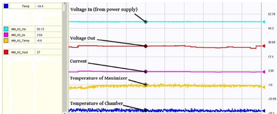
Figure 3: Smart-Curve function tested in thermal chamber for low temperatures
