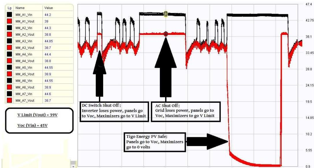
Figure 4: Smart-Curve response to system disturbance
